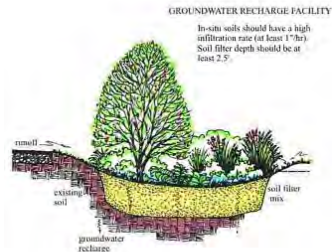
Diagram: Bioretention cells can either filter or filter and capture stormwater runoff. They use plants and layers of porous media to reduce quantity and improve the quality of stormwater runoff; connecting directly to existing stormwater structures. Low Impact Development Center, Inc., Beltsville, MD.
